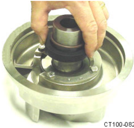
Figure 26 - Push Rotary Seal Down
