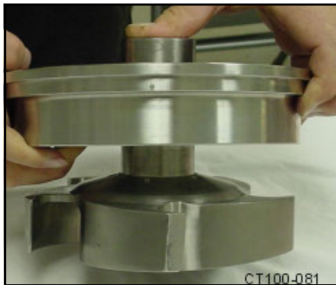
Figure 25 - Moving Rotary Seal Up the Shaft
