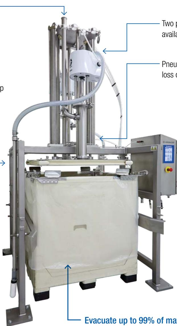
Two pump or four pump systems available with Graco piston pumps
