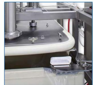
Inflatable wiper creates a tight seal preventing contaminants from entering the container
