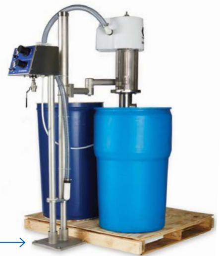
Stationary unit with base plate mounted to the floor
