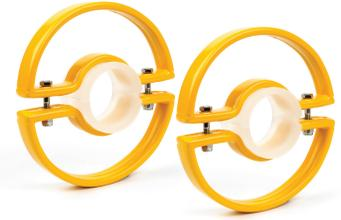
*The Golden Bridge is a heavy duty, safety yellow, hose support that easily bolts together over any hose or stainless steel piping system. A series of bridges elevate the hose or pipe off the floor keeping the hose clean, reducing wear and tear on the cover, and preventing damage to the sanitary end connections.*
