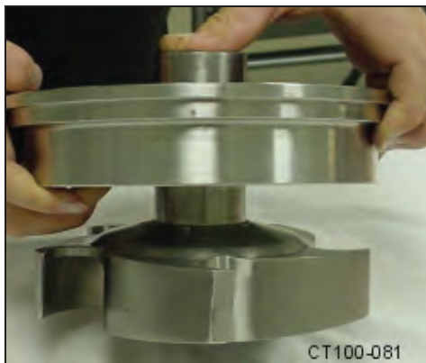
Figure 26 - Moving the Rotary Seal up the Shaft
