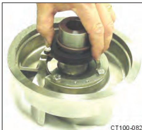
Figure 27 - Push Rotary Seal Down Until the o-ring is Released.
