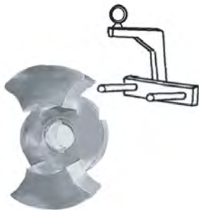
USE ROTOR REMOVAL TOOL TO REMOVE ROTORS
