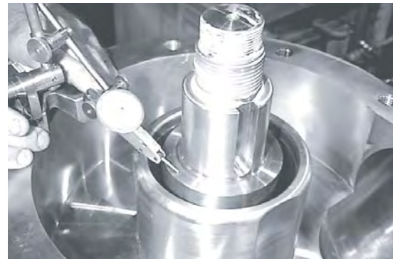
MEASURE DISTANCE BETWEEN HUB SHAFT SHOULDER AND ROTOR SHOULDER
