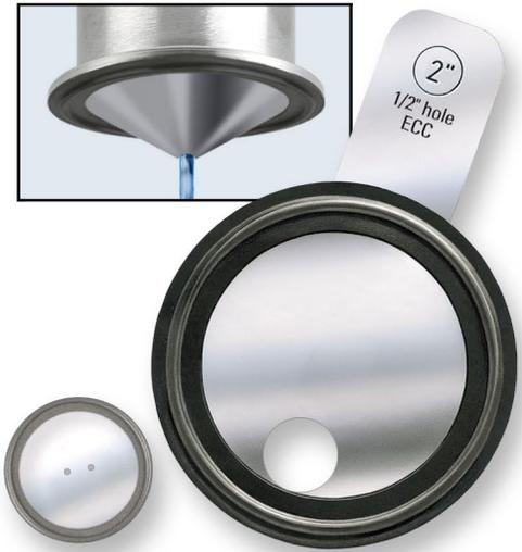
Our innovative Orifice Plate line includes a complete selection of solid 316L Stainless Steel, in standard or tabbed tri-clamp styles that can be custom drilled with an eccentric or concentric bore. Vertical styles, which are funnel shaped for optimal vertical drainage, are also available. Steam trap mini orifice plates are an alternative to standard steam trap technology.
