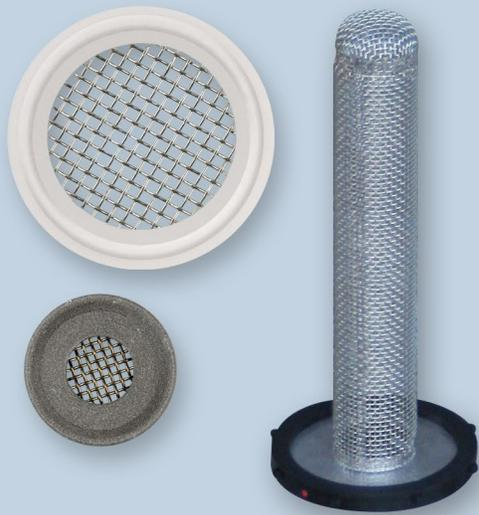
Rubber Fab's fluid filtration screen gaskets provide the most comprehensive range of stainless steel mesh and filter cloth. These gaskets provide particulate elimination to protect fill and finish sterile products, spray balls and spray nozzles. You can choose a screen gasket in a USP Class VI elastomer or Fluoroelastomer and are available in a variety of mesh sizes including 10 micron through 4 mesh. Custom screens are also available.
