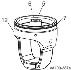
**Figure 17: Remove Yoke O-ring and Guide Bearing**
