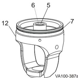
**Figure 28 : Remove Yoke O-ring and Guide Bearing**
