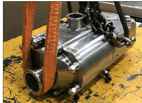
Figure 2 - Lifting location detail - 015, 030-UTS
