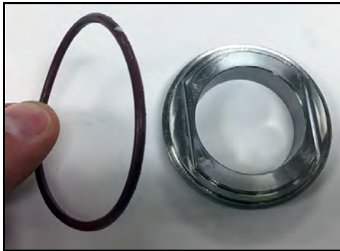
Figure 97 - Install cap-to-seat O-ring
