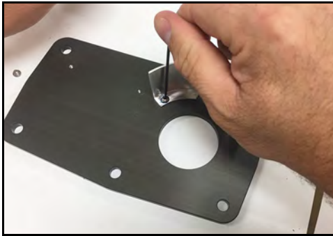
Figure 232 - Tighten shroud screws
