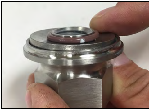
Figure 115 - Belleville washer installed
