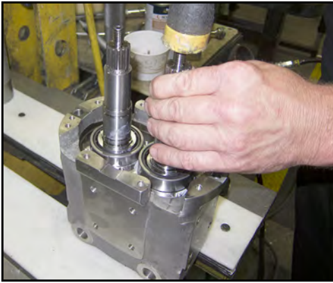
Figure 191 - Tap shafts to center in bores
