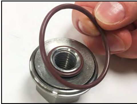
Figure 38 - Remove screw nut O-ring
