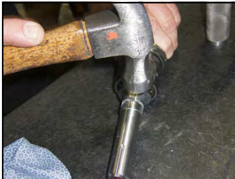
Figure 182 - Tap key into keyway
