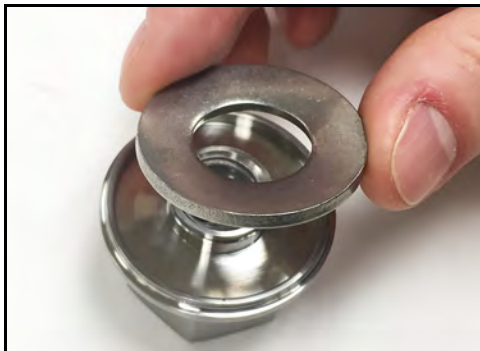
Figure 113 - Install belleville washer
