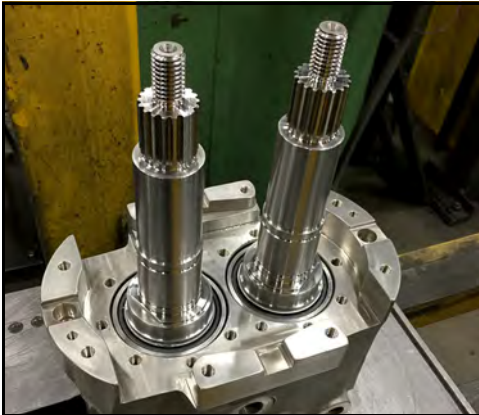
Figure 192 - Shafts seated in gearcase
