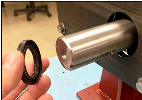
Figure 238 - Install oil seal
