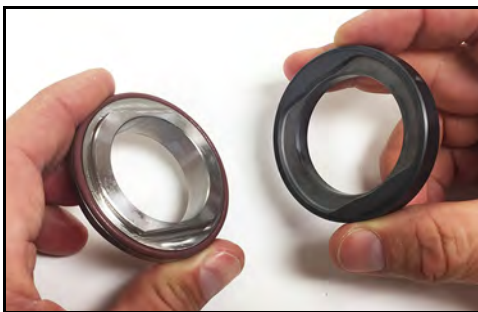
Figure 44 - Remove seal seat from seal cap
