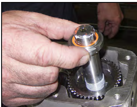
Figure 204 - Install locking nut
