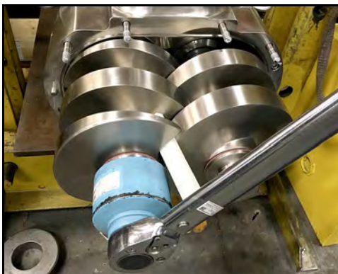
Figure 125 - Torque left screw nut
