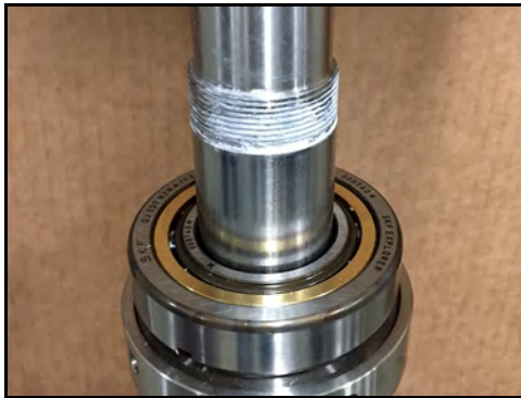
Figure 167 - Race installed on shaft
