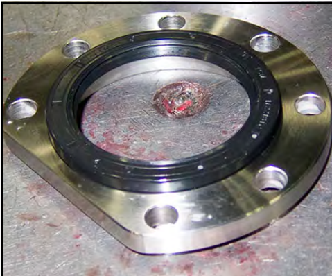
Figure 193 - Center bearing retainer seal
