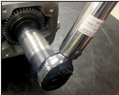
Figure 141 - Loosen locking nut
