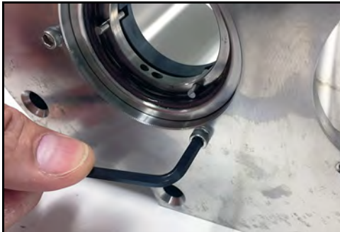
Figure 80 - Install with cap screws
