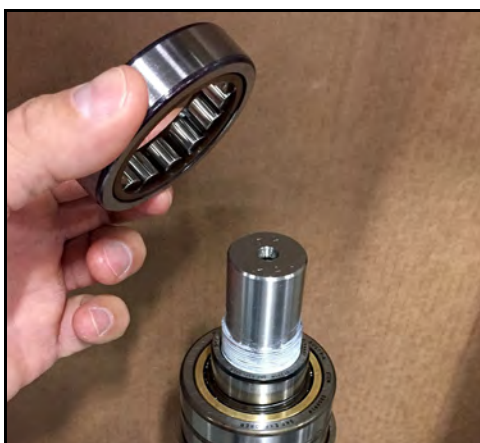
Figure 177 - Place bearing onto race
