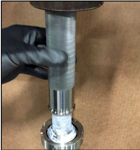
Figure 163 - Press race onto shaft
