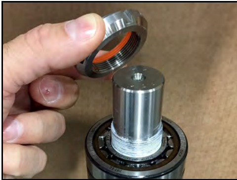
Figure 178 - Place locking nut onto shaft
