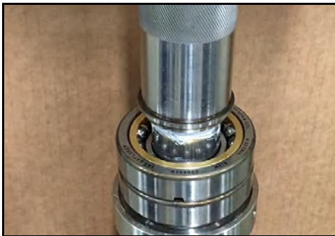
Figure 172 - Press race into bearing
