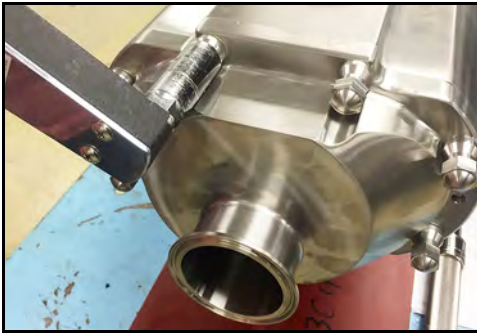
Figure 27 - Remove cover nuts
