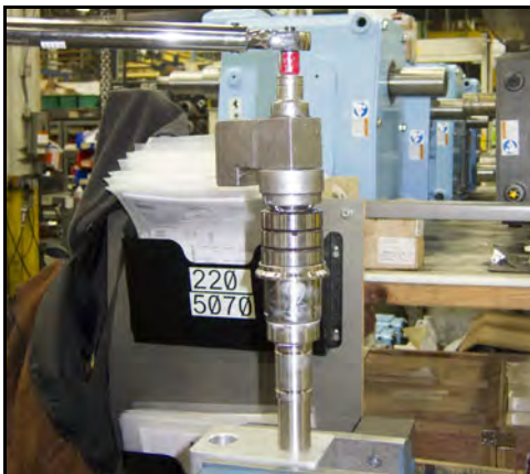
Figure 179 - Torque down locking nut
