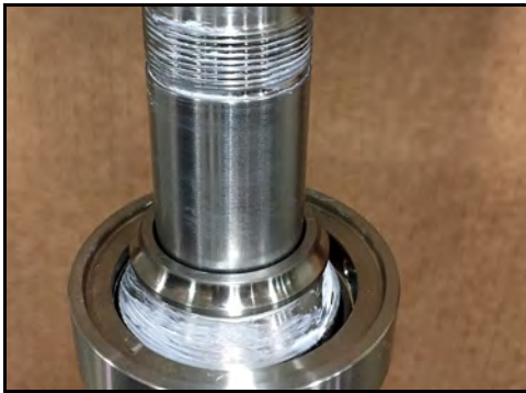
Figure 164 - Race pressed on shaft
