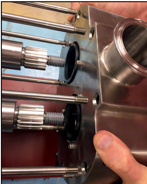
Figure 87 - Install pump body onto shafts
