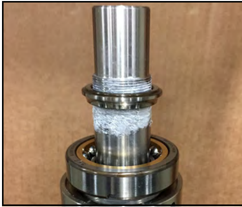
Figure 166 - Place race on shaft
