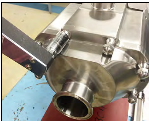
Figure 132 - Torque cover nuts
