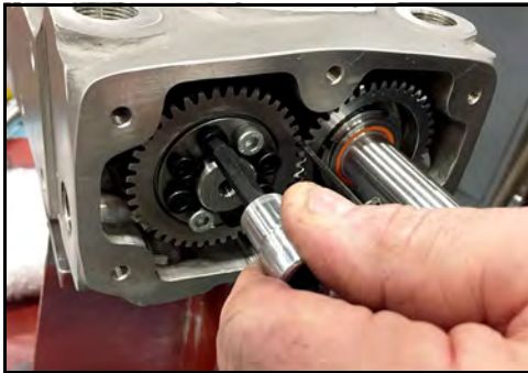
Figure 137 - Loosen bolts in locking assembly
