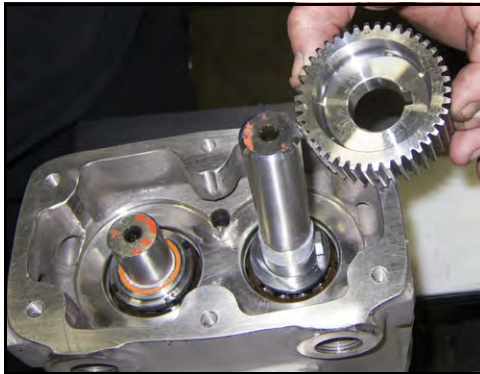
Figure 202 - Install drive gear
