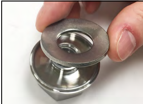
Figure 40 - Install Belleville washer
