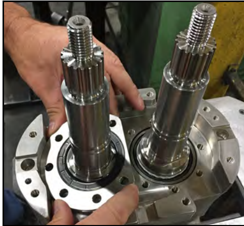
Figure 199 - Install bearing retainer
