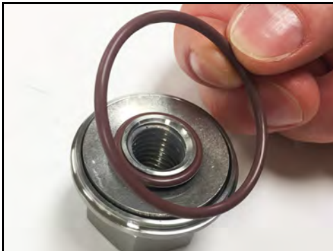
Figure 116 - Install screw nut O-ring
