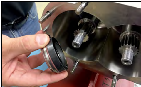
Figure 103 - Install seal cap assembly
