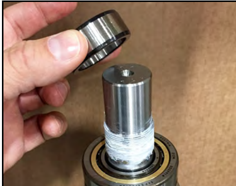
Figure 175 - Place race onto shaft
