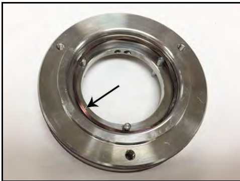
Figure 71 - Seal wave spring installed
