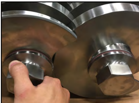
Figure 124 - Install screw nuts
