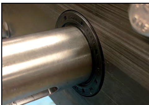
Figure 239 - Oil seal installed
