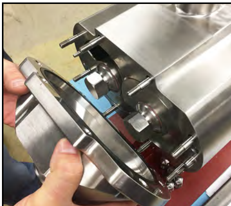
Figure 128 - Install pump cover
