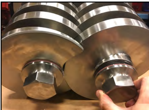
Figure 37 - Remove screw nuts
