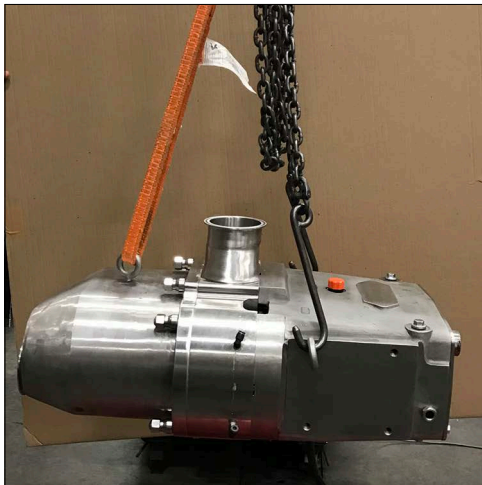
Figure 3 - Lifting location - 130, 220-UTS
