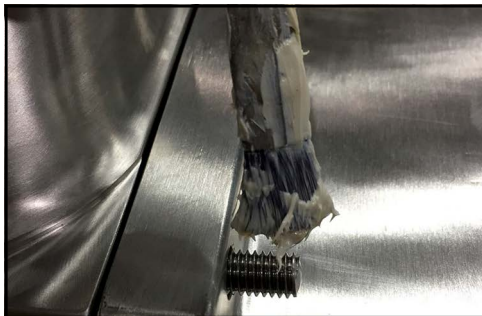
Figure 134 - Apply anti-seize to threads
