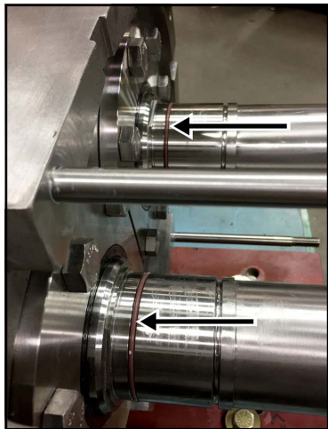
Figure 137 - Install shaft O-rings
