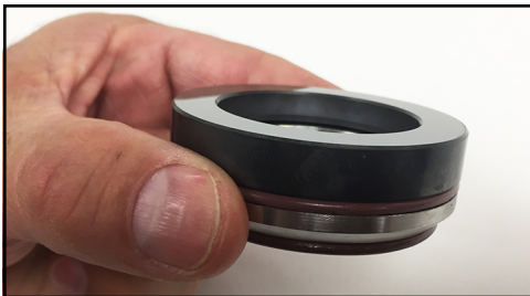
Figure 105 - Seal seat installed on seal cap
