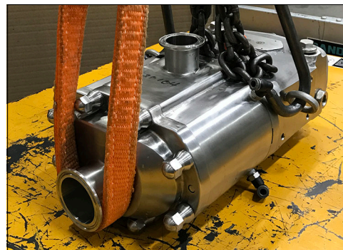
Figure 2 - Lifting location detail - 015, 030-UTS
