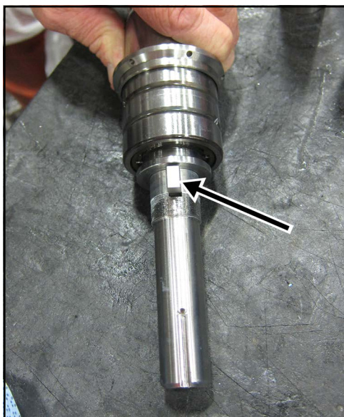
Figure 300 -Place key in key way
