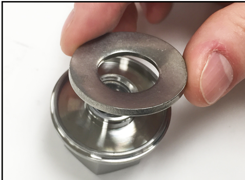
Figure 40 - Remove belleville washer
