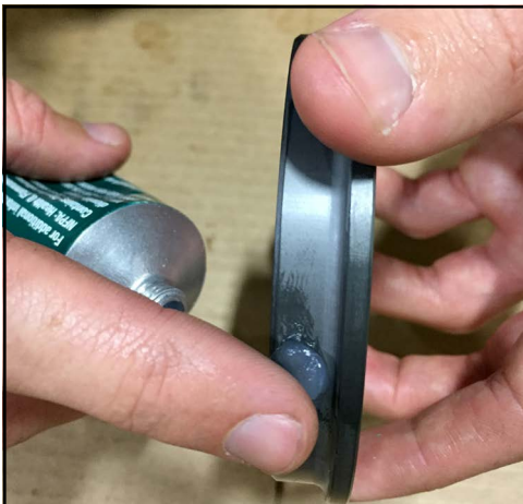
Figure 84 - Lubricate the outer diameter of the seal
