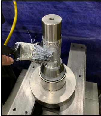
Figure 279 -Apply anti-seize to shaft
