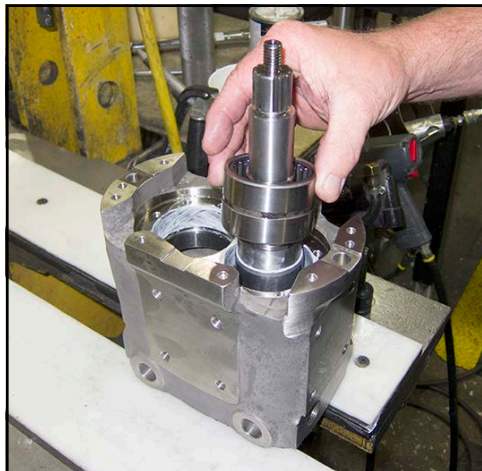
Figure 198 - Place outer race on shaft
