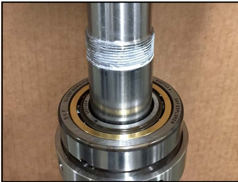
Figure 178 - Race installed on shaft
