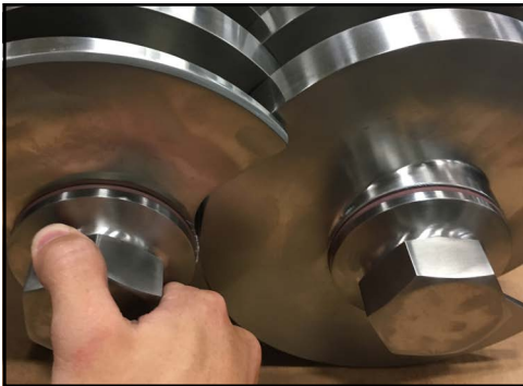
Figure 127 - Install screw nuts
