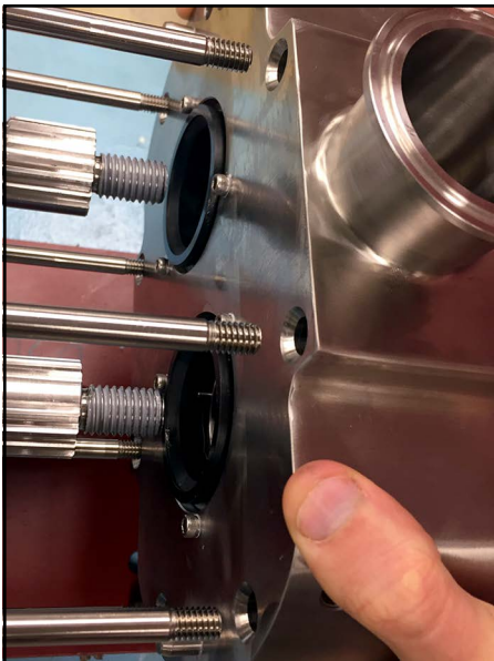
Figure 140 - -Install pump body onto shafts
