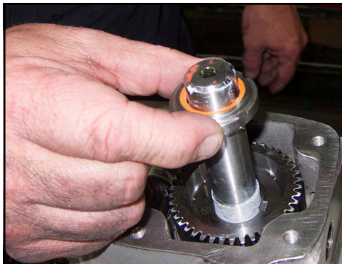
Figure 215 - Install locking nut
