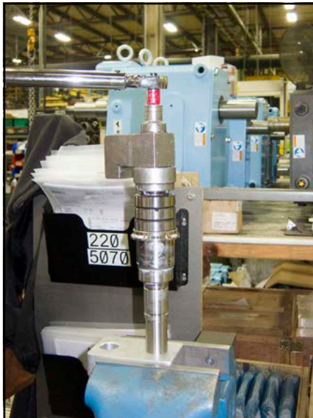
Figure 298 -Torque down locking nut
