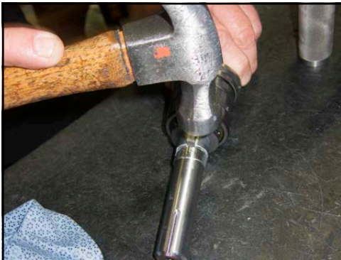
Figure 193 - Tap key into keyway
