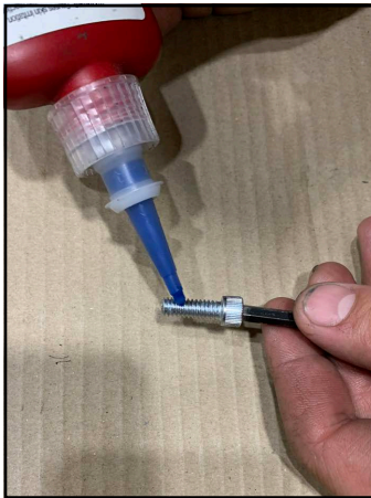
Figure 310 -Applying loctite Blue 242 to the rear bearing retainer bolts.
