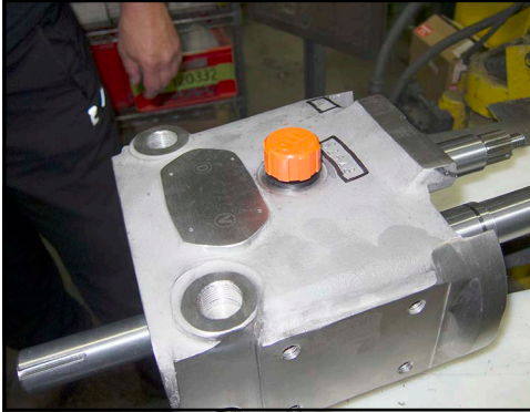
Figure 219 - Install oil breather plug
