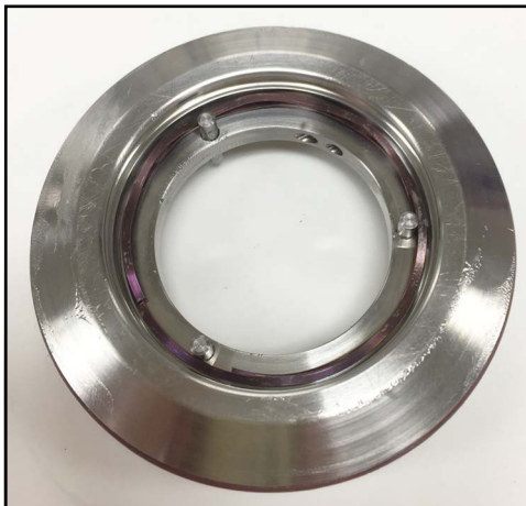
Figure 70 - Seal wave spring installed
