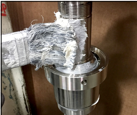
Figure 172 - Apply anti-seize to shaft
