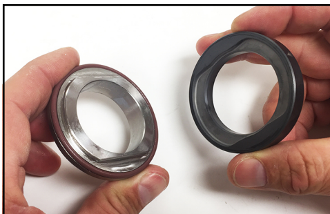
Figure 44 - Remove seal seat from seal cap
