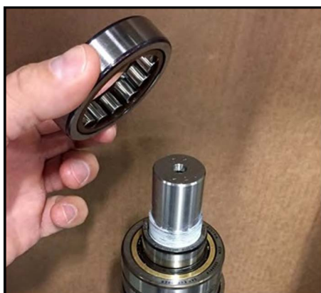
Figure 288 -Place bearing onto race
