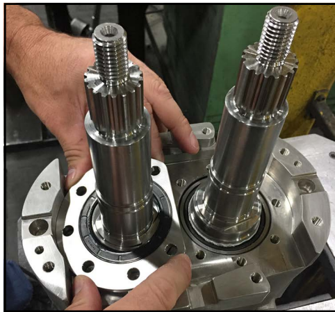
Figure 210 - Install bearing retainer
