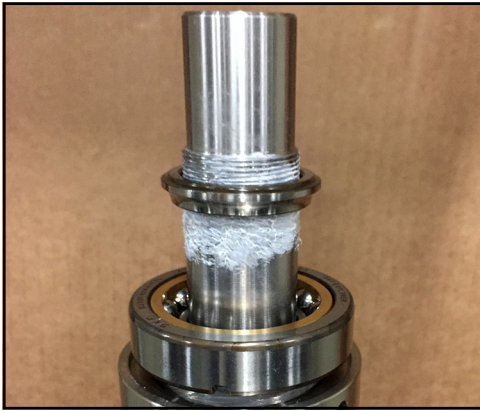
Figure 177 - Place race on shaft
