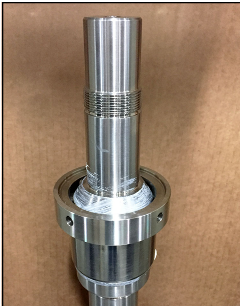
Figure 169 - Bearing spacer installed
