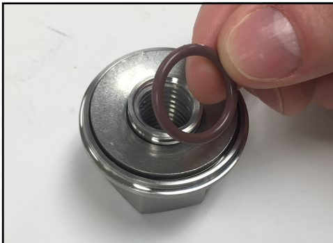
Figure 39 - Remove washer retainer O-ring
