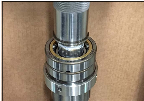
Figure 183 - Press race into bearing
