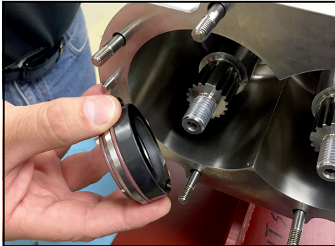
Figure 43 - Remove seal cap assembly
