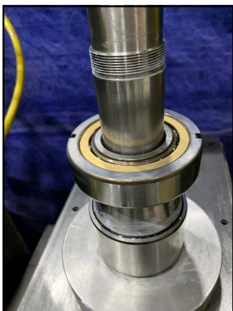
Figure 285 -Race installed on shaft
