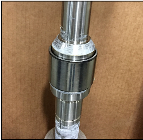
Figure 167 - Inner race installed on shaft
