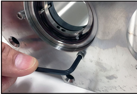
Figure 56 - Remove cap screws
