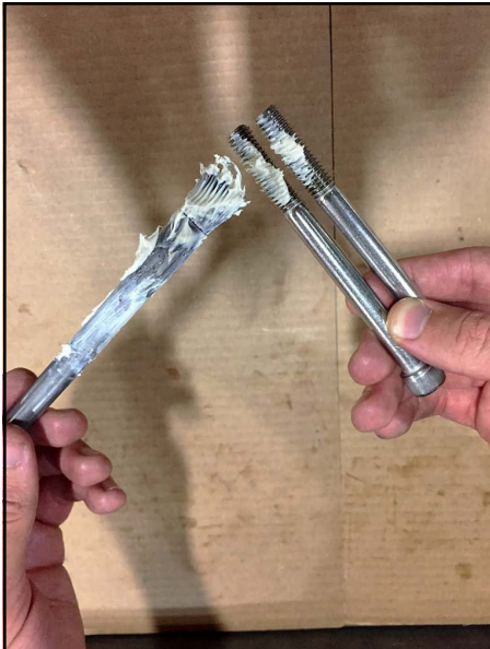
Figure 142 - Apply anti-seize to threads
