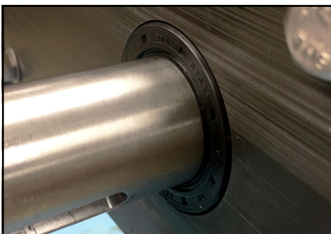
Figure 250 - Oil seal installed
