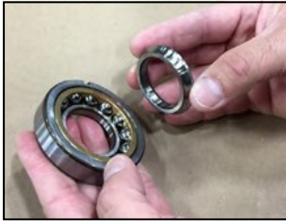
Figure 278 -Remove bottom race
