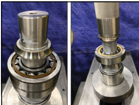
Figure 296 -Press race into bearing
