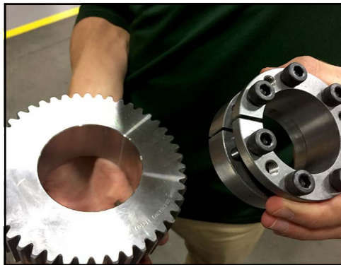
Figure 222 - Assemble locking assembly into gear
