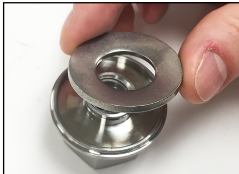
Figure 116 - Install belleville washer
