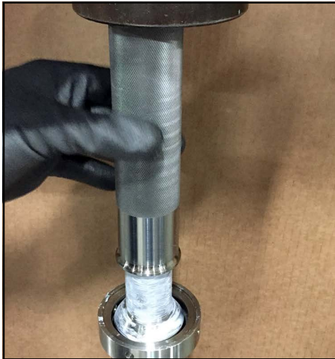
Figure 174 - Press race onto shaft
