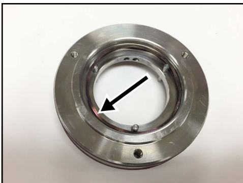
Figure 74 - Seal wave spring installed
