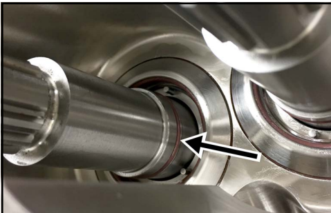
Figure 97 - Install shaft O-ring
