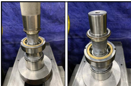
Figure 284 -Place race on shaft
