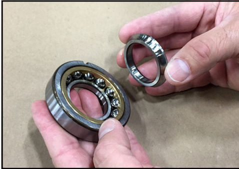
Figure 171 - Remove bottom race
