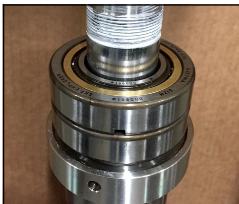
Figure 184 - Second bearing installed
