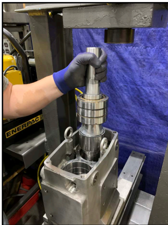
Figure 305 -Place drive shaft in bore
