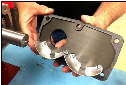
Figure 245 - Place gasket on cover
