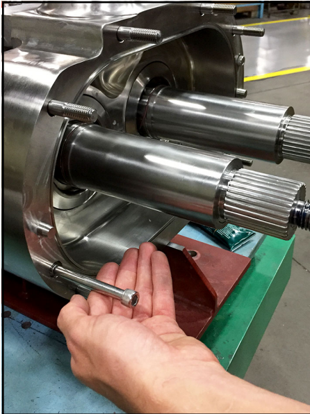
Figure 143 - Install body retaining screws
