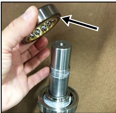
Figure 283 -Place bearing onto race
