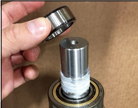
Figure 186 - Place race onto shaft
